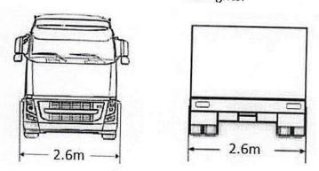
Note: Side cargo overhangs from the two sides of the vehicle cannot exceed 30cm.
